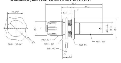
Suitable cable: MIL-TAC D 2 channel Ø 5.0 mm 4 channel Ø 5.5 mm Duplex 2 channel 2.8x5.5 mm 4 channel 2x 2.8x5.5 mm
