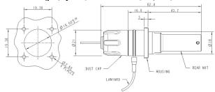
Suitable cable: MIL-TAC D 2 channel Ø 5.0 mm 4 channel Ø 5.5 mm Duplex 2 channel 2.8x5.5 mm 4 channel 2x 2.8x5.5 mm
