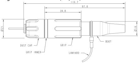
Suitable cable: MIL-TAC D 2 channel Ø 5.0 mm 4 channel Ø 5.5 mm
