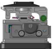
2. Slightly adjust the screw Right as shown. Clockwise to lift the blade, and vice in order to lower the blade height.
