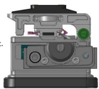
3. Open pressure fiberboard and cover plate, put bare fiber in the fixture that was stripped coating (125mm/900mm) ,press and close pressure fiberboard, push cutting block back and forth, then you can see the fiber cleaver's blade whether just meet fiber or not ,if not, please repeat step 2.Lift blade, if meet too much, please repeat step 2 to lower blade.
